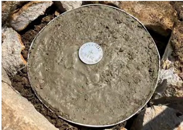
Photo Orientation & Description: Capped rebar in concrete
