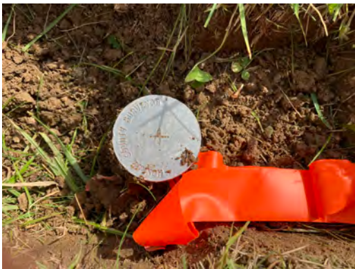
Photo Orientation & Description: Capped rebar at E11
