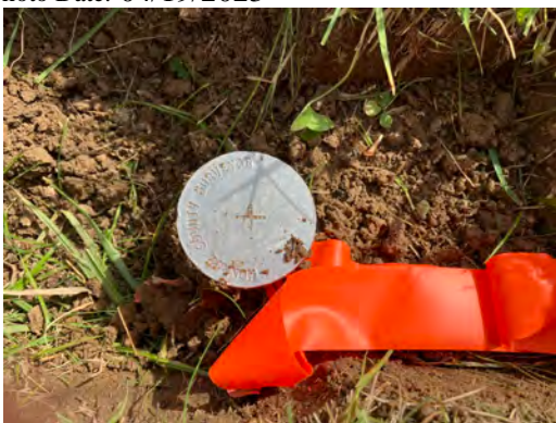
Photo Orientation & Description: Capped rebar at E11
