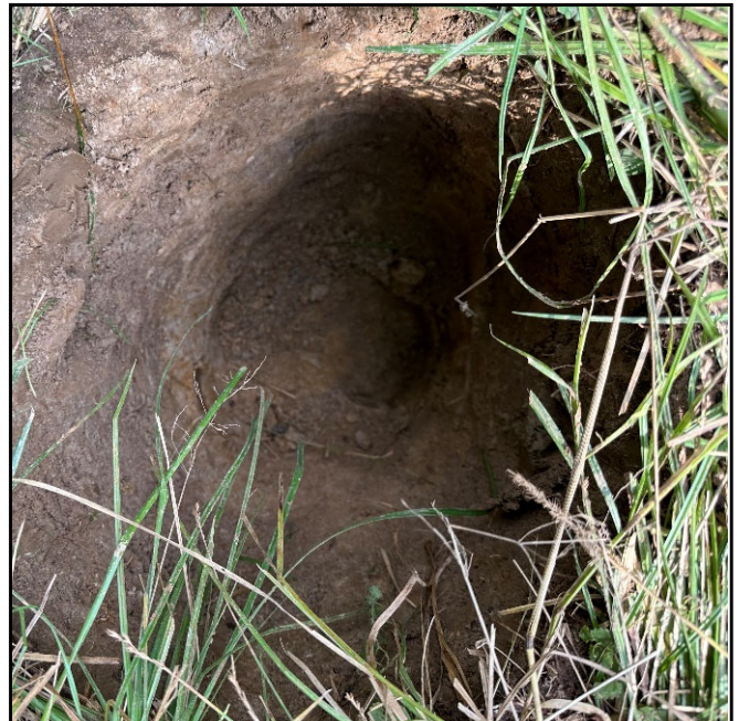
Photo 8: DP-2 Test Pit showing absence of soil saturation; View down
