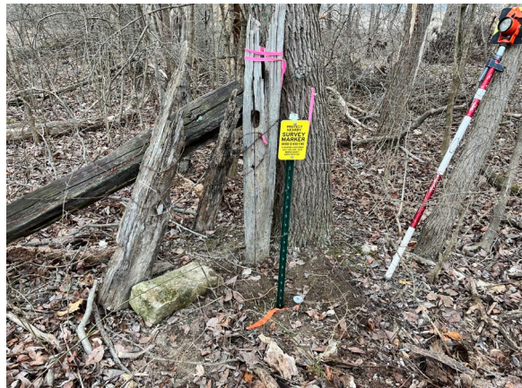
Photo Orientation & Description: From Southwest looking Northeast, showing rebar set and engraved stone found lying on ground.
