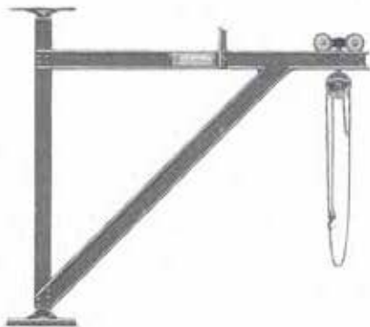
Type 2—Underbraced Jib Crane \frac{1}{2} to 2-ton capacity
