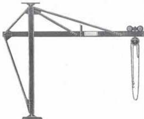
Type 4—Top and Backbraced Jib Crane 2 to 10-ton capacity
