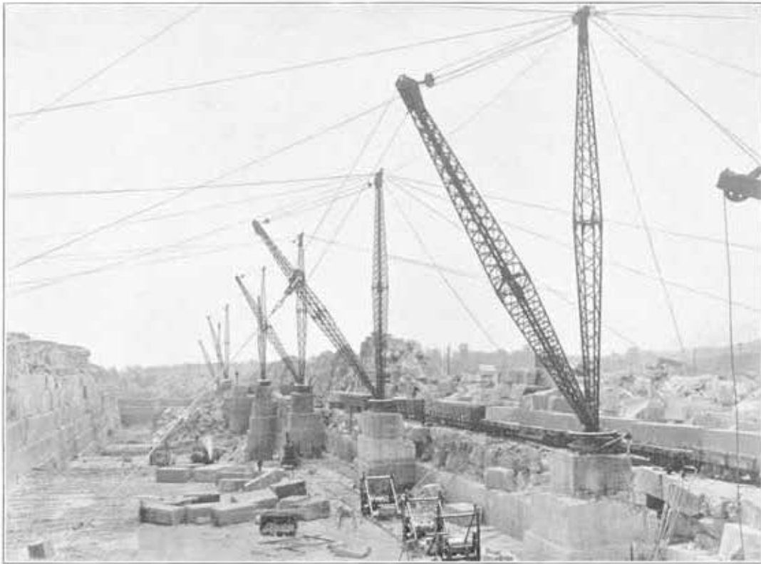
Typical Quarry Scene, showing Number of Steel Derricks and Bedford Electric Channelers
